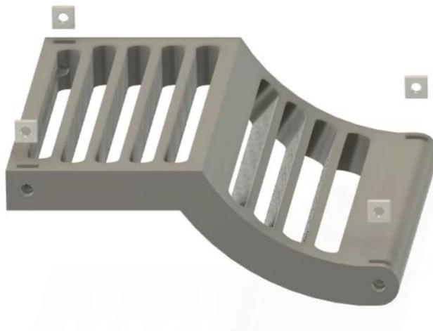
This step is very simple. We insert 4 square nuts into the cross plate and fix them if necessary.
