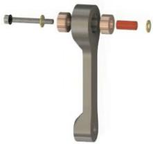
Next, we assemble the lever. We insert the two ball bearings flush and push the nozzle through the bearings. Insert an M3x20 screw with 2 washers (as shown) through the nozzle.
