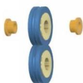
If possible, these should be printed from flexible material. We now place the two tires (e) on the 10 mm mini ball bearings. Then insert the two bearing caps (h) into the upper bearing. Now insert the two bearing caps (d) onto the lower bearing from both sides. This also fixes the upper bearing, which can still move freely in the slotted hole groove.
