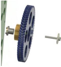
Now insert the ZDR at an angle to the already installed small Z2L, pull out the bearing bush at a slight angle and carefully lever the gearwheel and bearing onto the bearing bush until the gearwheel is seated and firmly hooked in with Z2L across its entire width. This can be a little fiddly.
