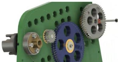
At the same time, we must place the gearwheel **Z3L** (c) against the side of the intermediate gearwheel **ZDR** from behind. The labelling must be legible.
