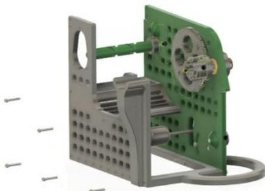
Firstly, we place the front plate on the base plate and make sure that the cross plate also engages in the pre-milled groove. We also make sure that the double helix protrudes into the keyhole-shaped hole.
