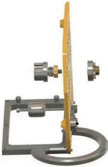
The two **parts A & B** are now firmly connected in the centre plate via the ball bearing with the M3x30 screw. The screw is screwed into the nut (c), which is clamped in the flange plate (d).
