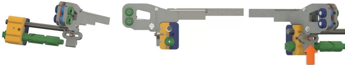
Finally, we slide the filament guide with the dovetail groove onto the tab and fix it in the center with an M3x8 screw including an M3/7 washer.
