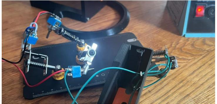
Then we solder the reverse switch according to the circuit diagram, first a1, b2 and b1 b2 crosswise, then the connections to (a) and (c). We solder the two cables or 4 wires to the sensors, i.e. to the jack sockets, to the switches and lead them out from the inside to the outside. Polarity and sensor position are not important as the sensors are connected in series.
