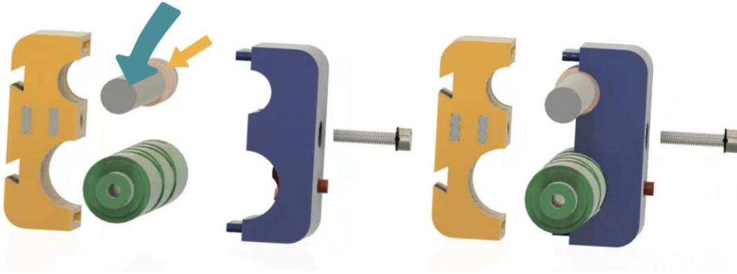
To do this, we push the two built-in plain bearings into a central position on the rail and then push the rider part shown in blue onto the two plain bearings. Make sure that the T piece is positioned correctly and is placed in a thread of the double helix. We press both rider parts together. When there is no longer a visible gap and they can no longer be pushed back and forth on the helix, we can screw them together.
