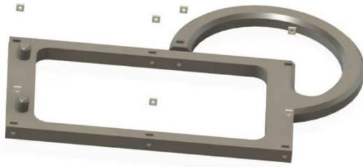
Next, we prepare the base or floor plate. Insert 7 M3 square nuts and, if necessary, fix them with a piece of tape until they are needed.
