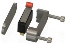
The button prepared in this way is inserted into the button housing. The front screw (M3x20) is screwed into the nut that has already been pressed in. The second screw (M3x20) is inserted through the bend and secured from the inside with a washer and nut. The sensor is later adjusted via this bend.
